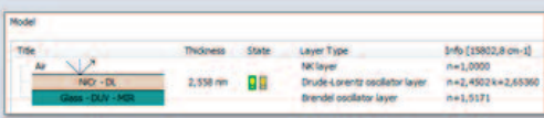
Fig. 3: Optical model description of the single layer thin NiCr film on clear float glass.
